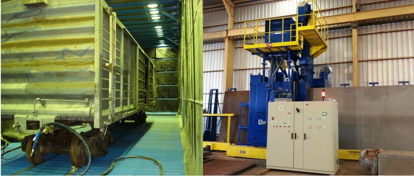
Shot blast production lines, both manual and automated systems, became possible with the introduction of centrifugal wheel blast machines. The system of shot blasting by centrifugal wheel is more productive than by compressed air and achieves a better more uniform surface finish.
